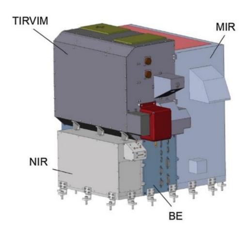
Fig.1 The atmospheric chemistry suite comprises four units: the NIR, MIR, and TIRVIM spectrometers and the electronic block (EB). Image courtesy of the researchers. Credit: Researchers 10.1007/s11214-017-0437-6
