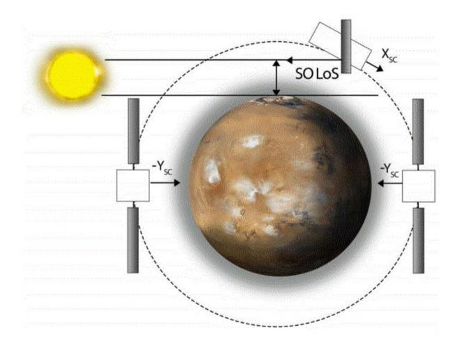
Fig. 2. Three observation modes of the Trace Gas Orbiter: the so-called solar occultation measurements (top right) of light passing through the Martian atmosphere and nadir, or "straight-down," measurements of reflected sunlight and Mars' own radiation from its dayside (left) and nightside (right). Credit: Researchers 10.1007/s11214-017-0437-6
