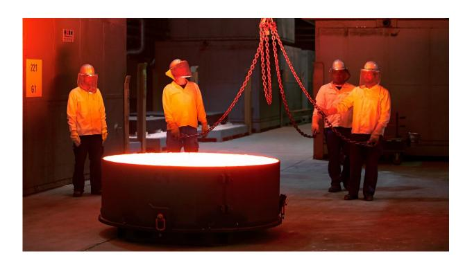
The first hexagonal segments for the main mirror of ESO's Extremely Large Telescope (ELT) are shown being successfully cast by the German company SCHOTT at their facility in Mainz. These segments will form parts of the ELT's 39-metre main mirror, which will have 798 segments in total when completed. The ELT will be the largest optical telescope in the world when it sees first light in 2024. Credit: SCHOTT/ESO
