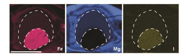
The diamond anvil cell recreated the conditions of early Earth as the material that's analogous to the core -- inner dashed line -- separates from the material that's analogous to the magma ocean in the mantle--the outer dashed line. The scale bar in the left panel is 10 microns. Credit: Colin Jackson.
