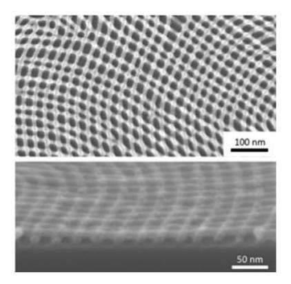
Plan view (top) and cross-sectional (bottom) scanning electron microscope images of an inorganic nanomesh created through iterative self-assembly and infiltration synthesis. Credit: Gregory Doerk
