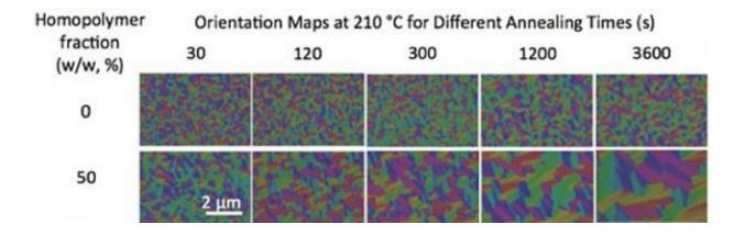
Without blending, the size of grains (single-color regions) of a diblock copolymer with a molecular weight of 36 kilograms/mole barely changes with thermal annealing over time (top row). Blending the block copolymer with homopolymers increases the grain size and speeds up the ordering process (bottom row). Credit: Gregory Doerk
