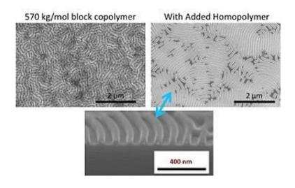
A comparison of scanning electron microscope images after solvent vapor annealing of a large block copolymer (top left) and the same copolymer with added homopolymer (top right) shows that the homopolymer can significantly improve pattern quality. The bottom image is a cross-sectional image of the top right sample. Credit: Gregory Doerk
