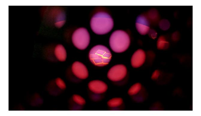
Diamond plates undergoing surface termination treatment in a hydrogen plasma. Credit: Daniel Creedon
