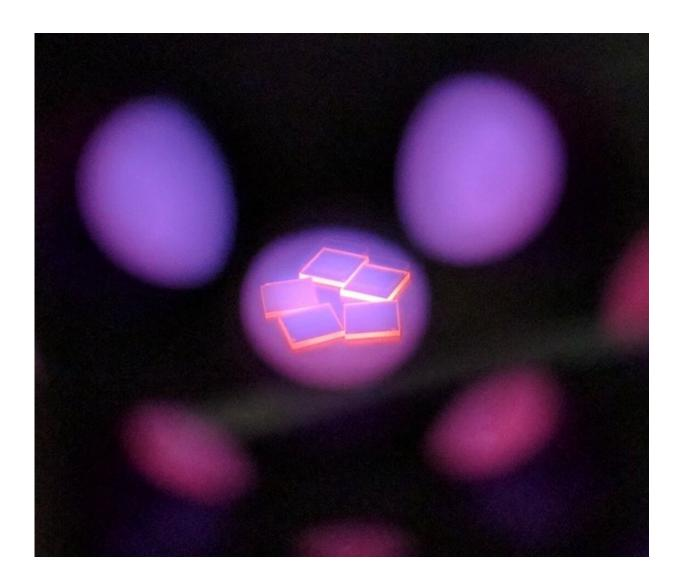
Diamond plates undergoing surface termination treatment in a hydrogen plasma. Credit: Daniel Creedon
