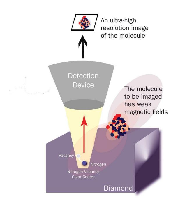
Researchers led by Nathalie de Leon are turning diamonds into devices that can image single molecules. The device uses a defect in the crystal structure called a nitrogen-vacancy color center. When disrupted by the molecule's faint magnetic field, the defect gives off red signals that can be used to construct an ultra-high resolution image of the molecule. Credit: Yasemin Saplakoglu
