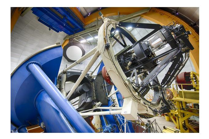
The Dark Energy Camera is mounted on the Blanco telescope in Chile. Credit: Fermilab
