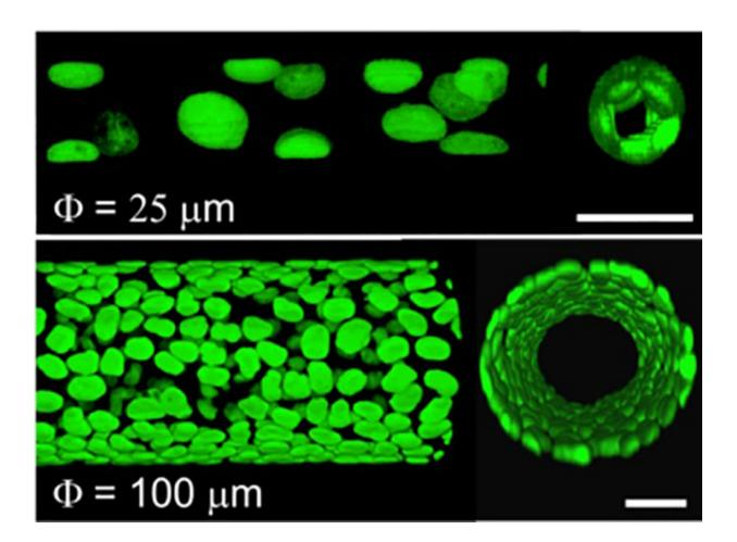
The arrangement of cells into lumen-containing structures inside polydimethylsiloxane (PDMS) microtubes with varying diameters (25 microns and 100 microns). Credit: Mechanobiology Institute, Singapore
