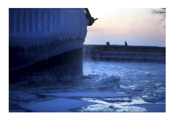
Steam rises from Lake Superior as the ship St. Clair comes to harbor during some of the coldest temps of the year, Sunday, Dec. 31, 2017, at Canal Park in Duluth, Minn. The St. Clair is a self-unloader built in 1976 at Sturgeon Bay, Wis., and is 770 feet long and has 26 hatches that open into 5 cargo holds, providing a load capacity of 45,000 tons. (David Joles/Star Tribune via AP)
