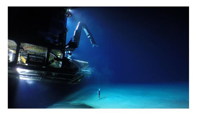
The remotely operated vehicle (ROV) Jason lands on the seafloor at Havre submarine volcano to retrieve a heat flow monitor. Credit: Multidisciplinary Instrumentation in Support of Oceanography (MISO) Facility, ©Woods Hole Oceanographic Institution
