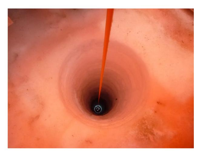
A team of ice drillers from Victoria University of Wellington used hot water and a drilling system developed at Victoria to melt a hole through hundreds of metres of ice. Credit: Craig Stevens, CC BY-ND
