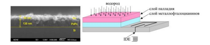
Photograph of the layers of palladium and phthalocyanines on the surface of the electrode, obtained with the help of a scanning electron microscope (left). A schematic image of the sensor (right). Credit: Pavel Krasnov
