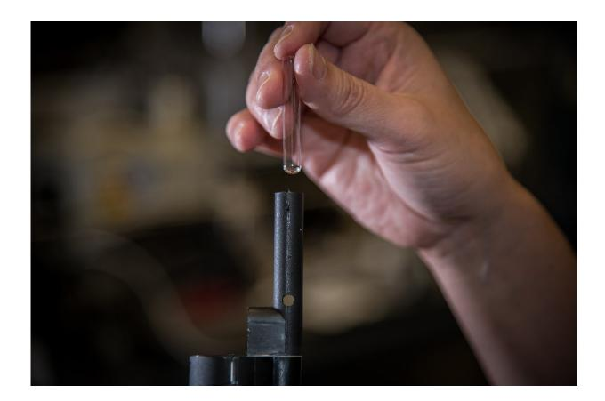
An ampule of chemical simulant, meant to imitate the deadly chemicals used in warfare, is loaded into the Threshold Confidence Checker. Credit: Jason Stoughton/NIST
