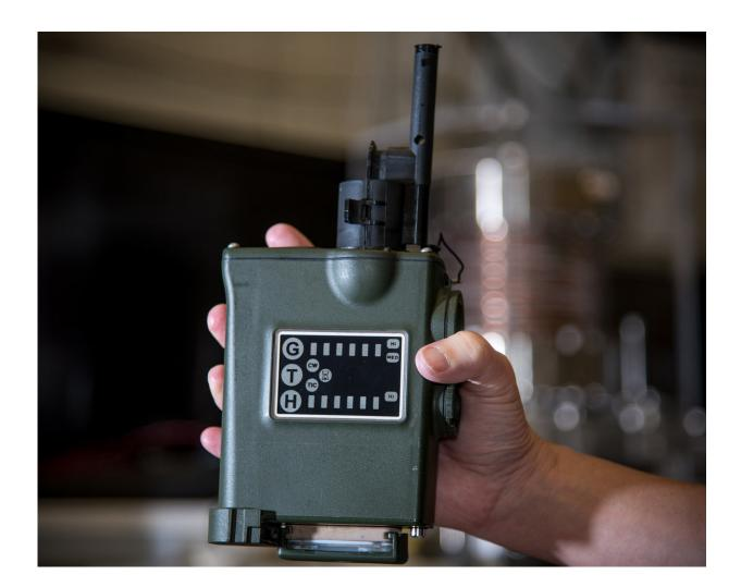
A Joint Chemical Agent Detector equipped with a threshold confidence checker in black, on top. Credit: Jason Stoughton/NIST
