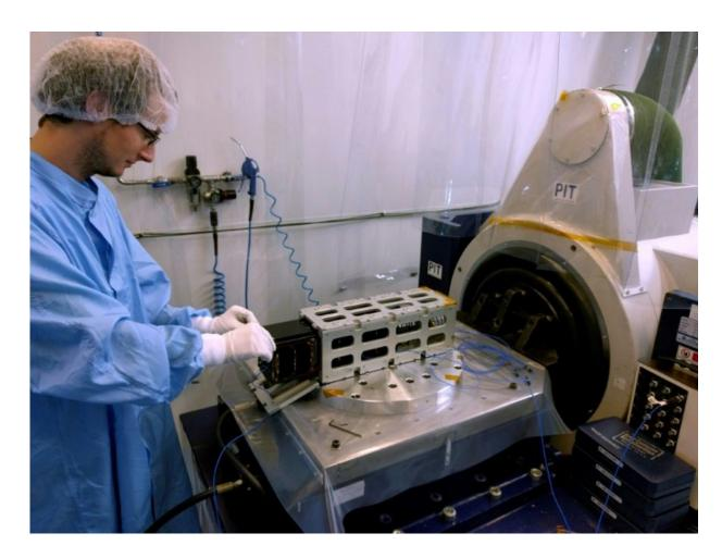
System manager Lester David puts the PicSAT Flight model in its launch pod for testing on the vibration table in Saint-Quentin-en-Yvelines
