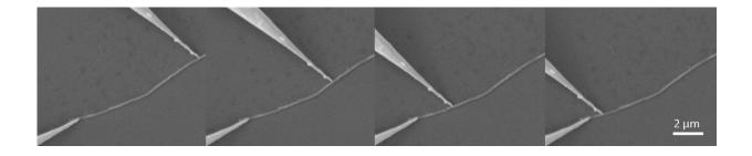
Scientists at Rice and Swansea universities used tungsten probes attached to a scanning tunneling microscope to test the conductivity of carbon nanotubes before and after treatment to decontaminate them. The sequence above shows one probe at the end and the other moving along the length of an isolated nanotube. Credit: Barron Research Group/Rice University
