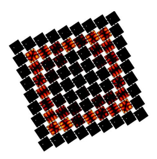
An illustration of a metamaterial designed by Daraio's team. Though each individual square is identical, their layout and the metamaterial's overall design cause waves to propagate in a specific pattern through the material, as indicated by the squares' different colors. Credit: Chiara Daraio/Caltech
