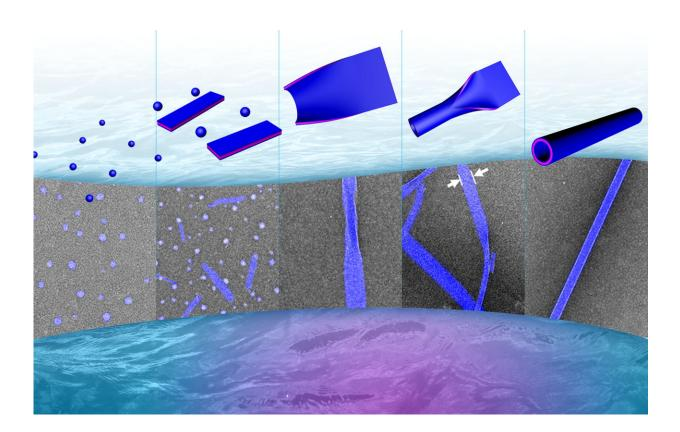
Scientists at PNNL have created a new family of nanotubes that are composed of peptide-like molecules called peptoids. These nanotubes start out as small droplets that come together to form a cell-membrane-like sheet. Then the sheet folds at one end and zips closed into a tube. Credit: PNNL
