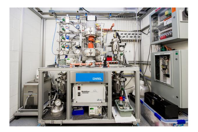
The catalytic reactor shown here is for converting chemical intermediates into acrylonitrile. The work is part of the Renewable Carbon fiber Consortium. Credit: Dennis Schroeder/NREL
