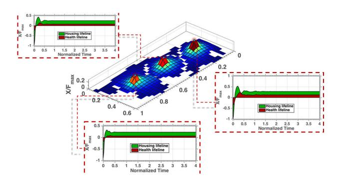
A map of Gotham City is laid out in a Finite Element Analysis grid. The grid shows how stresses to different lifelines affect various parts of the city. Credit: Colorado State University
