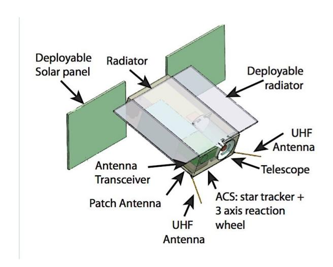
The SPARCS space telescope is CubeSat that will be built at ASU out of six cubical modules, each about four inches on a side. The plan is for students to be involved the design and construction of the spacecraft to provide educational and training opportunities to become future engineers, scientists, and mission leaders. Credit: Arizona State University
