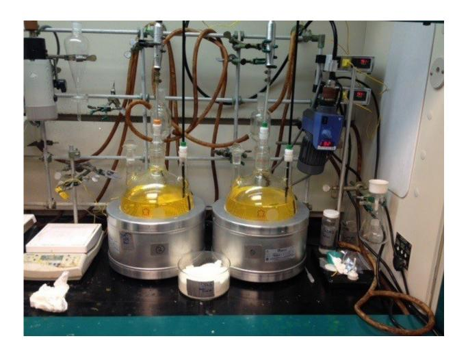
Diaminoglyoxime is shown in the foreground, following filtration and drying from the reaction mixture. In the background, DAG is being synthesized in a pair of 500 gram scales. Credit: Eric C. Johnson
