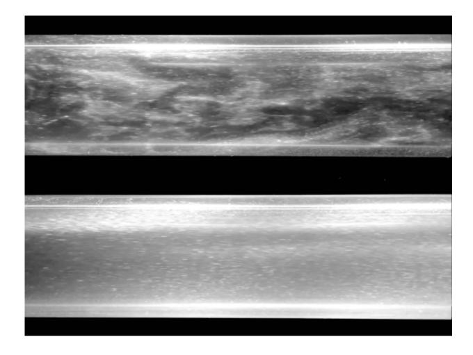
Turbulent flow (top) compared to laminar flow (bottom). Credit: Jakob Kühnen
