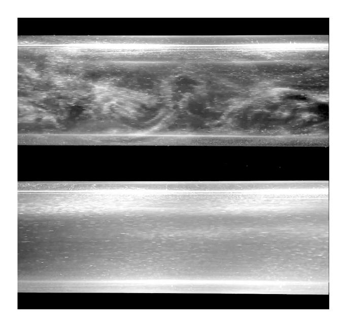
Turbulent flow (top) compared to laminar flow (bottom). Credit: Jakob Kühnen
