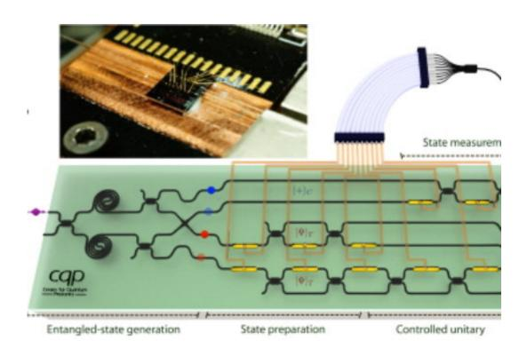
Rendered pictorial representation of the photonic chip designed and used for the experiment, along with a description of the essential instruments employed. A schematics of the working principle and steps of the algorithm is also superimposed. Inset - a photo of the chip, mounted on the circuit board used as interface. Credit: University of Bristol
