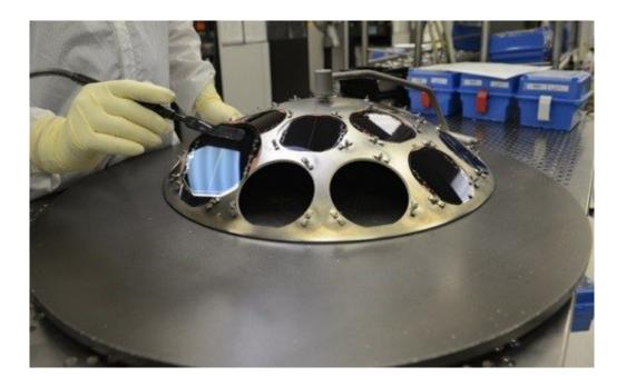
Inverted Metamorphic Multi-Junction (IMM) Solar Cells are a more efficient and lighter weight alternative to the state-of-practice multi-junction space solar cells. A collaboration between the Air Force Research Laboratory, the U.S. government and industry has led to refinement of the IMM solar cell growth process, ensuring high yield, efficient solar cell production through industrial manufacturing optimization. Credit: SolAero Technologies
