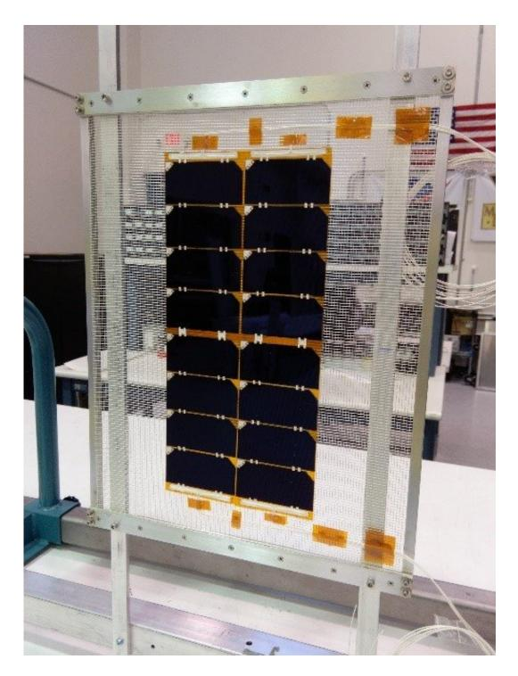
Inverted Metamorphic Multi-Junction (IMM) Solar Cells are a more efficient and lighter weight alternative to the state-of-practice multi-junction space solar cells. A collaboration between the Air Force Research Laboratory, the U.S. government and industry has led to refinement of the IMM solar cell growth process, ensuring high yield, efficient solar cell production through industrial manufacturing optimization. Credit: SolAero Technologies
