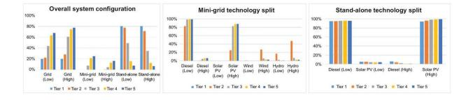
Overall system configuration (left); mini-grid technology choice (middle); standalone technology choice (right) for low and high diesel prices and fro 5 tiers of electricity consumption. Credit: European Commission, Joint Research Centre (JRC)
