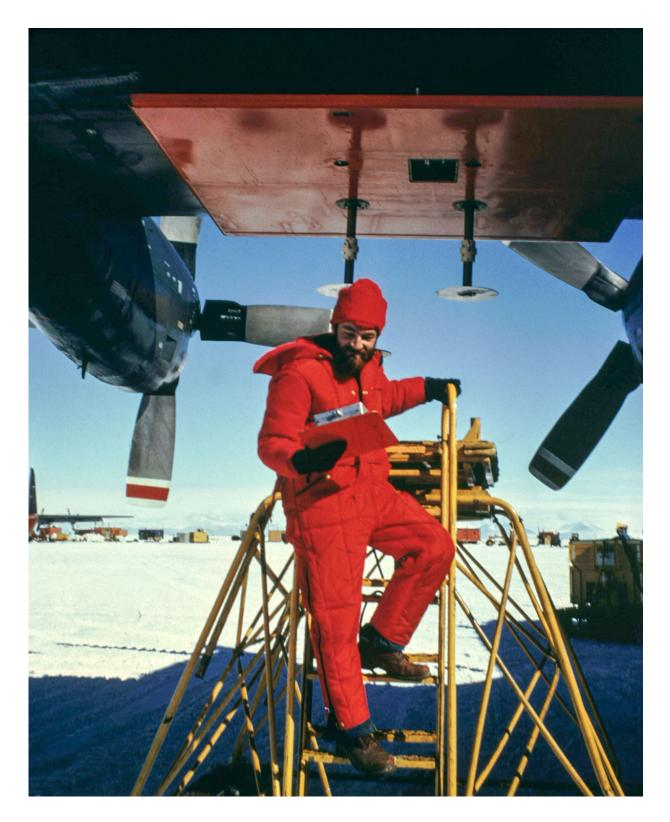
Nils Sko undertaking maintenance on a 300MHz radar antenna on a C-130 plane at McMurdo Sound in Antarctica. Credit: Courtesy SPRI
