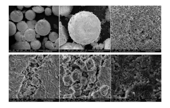
SEM images of the porous surface at increasing microscopy strength (from top left). Credit: KAUST
