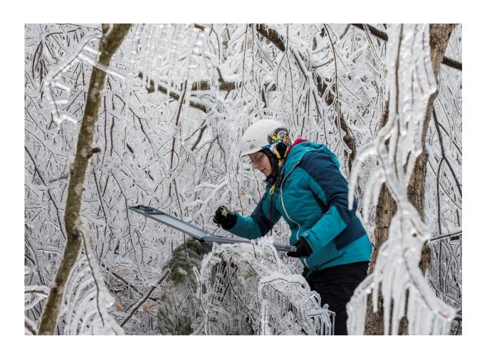
Wendy Leuenberger, a former graduate student at SUNY-ESF, measures ice accumulation following a simulated ice storm at the Hubbard Brook Experimental Forest, NH. Credit: Joe Klementovitch
