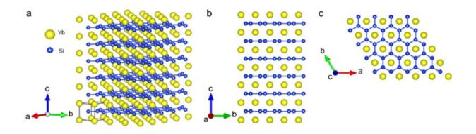
(a) Three-dimensional crystal structure of YbSi2, (b) view along the a-axis, and(c) along the c-axis. Credit: 2017 Kurosaki et al. Phys. Status Solidi RRL 2017, 1700372. doi: 10.1002/pssr.201700372
