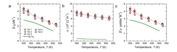
Temperature dependences of (a) the Seebeck coefficient S, (b) electrical
