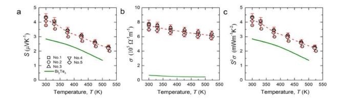
Temperature dependences of (a) the Seebeck coefficient S, (b) electrical
