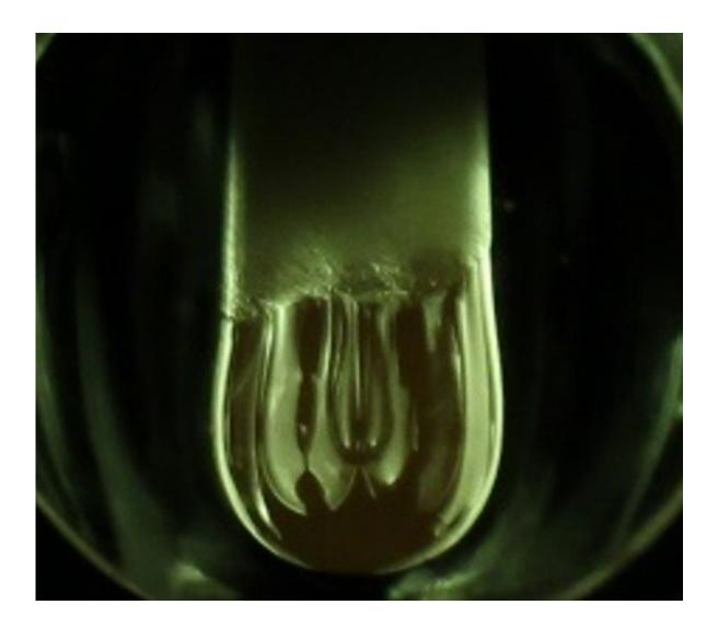
A molten hanging droplet, or pendant (at center), forms from an aluminum oxide rod under intense heat and light from xenon lamps. Using this process, MIT researchers have demonstrated a new electrochemical method to study thermodynamic processes in a molten oxide melt at temperatures above 2,000 degrees Celsius. Credit: Melody M. Wang
