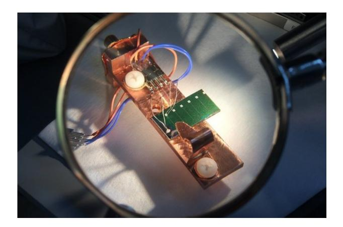
This experimental setup was used by the team to measure the electrical output of a sample of solar cell material, under controlled conditions of varying temperature and illumination. The data from those tests was then used as the basis for computer modeling using statistical methods to predict the overall performance of the material in real-world operating conditions. Credit: Riley Brand
