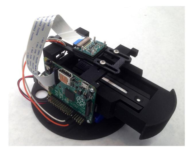
The TIDBIT reader overview showing components and internal structures of the device. Credit: *PNAS*
