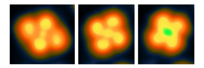
The images from the scanning tunnelling microscope (STM) show the three different states of the molecule, which correspond to a trinary code for encrypting information: in a highly magnetic state (left), in a low magnetic state with atoms that have moved closer together (middle) and in an equally low magnetic state but turned by 45 degrees (right). Credit: Manuel Gruber
