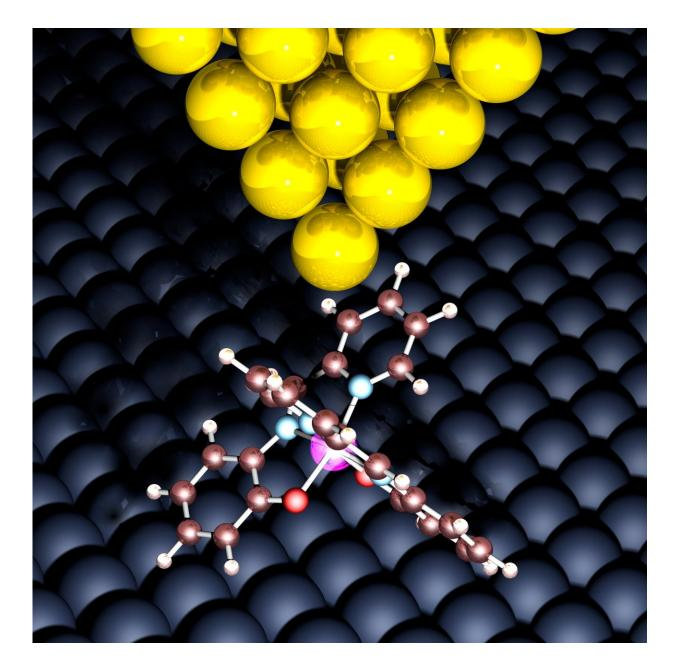
The tip of the STM (yellow) assumes the role of a hard drive's reading and writing head for the molecule attached to the copper nitride surface (black). Credit: Manuel Gruber
