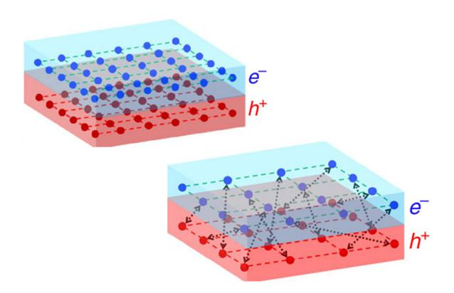
Rice's "topological excitonic insulators" are made of sheets of semiconductors (top) that become insulators at a critical temperature around 10 kelvins. At the critical point, a superfluid quantum liquid of excitons -- pairs of negatively charged electrons (blue dots) and positively charged electron holes (red dots) -- forms inside the devices (bottom) and electricity ceases to pass through them. Credit: R. Du/Rice University
