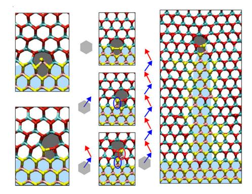
A slight mismatch between the hexagonal structures of molybdenum disulfide and tungsten diselenide creates a strain that can be released by the formation of a "517 dislocation," in which two hexagons collapse to form a pentagon and a heptagon. Reactions with molybdenum disulfide in the environment cause the dislocation to move deeper into the tungsten diselenide, drawing a nanowire of molybdenum disulfide behind it. Credit: Massachusetts Institute of Technology
