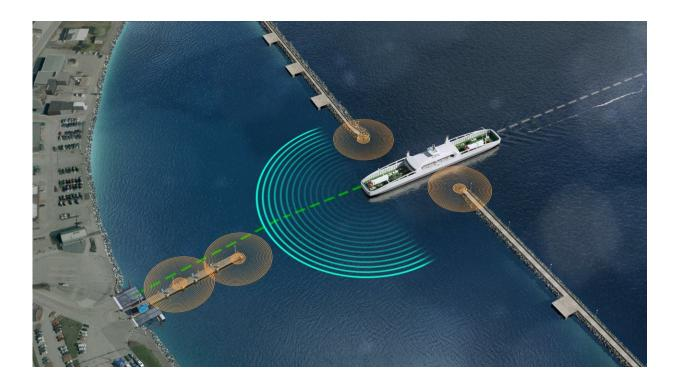
An autodocking system automates the first and last phases of the crossing right up to the quay. Autodocking systems use additional sensors to assess proximity to harbour structures such as moles at the entrance, and distance to the berth. The propulsion system is adjusted by the system to bring the ferry safely and with minimum energy consumption to and from the docks. Credit: Rolls-Royce Plc
