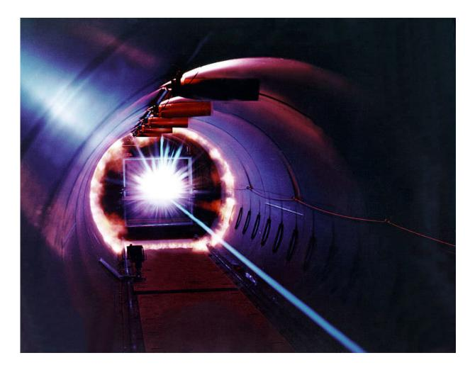
The interior of the Hypervelocity Ballistic Range at NASA's Ames Research Center. This test is used to simulate what happens when a piece of orbital debris hits a spacecraft in orbit. Credit: NASA/Ames
