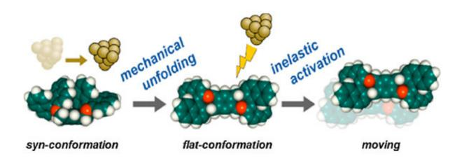
Schematic diagram showing the interaction of tunneling current with molecules. Credit: National Institute for Materials Science
