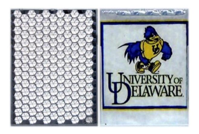
Researchers created a prototype smart glass that is retroreflective (left) and becomes clear (right) when a liquid with optical properties similar to the reflective structure is pumped into a chamber in front of the structure. Credit: Keith Goossen, University of Delaware
