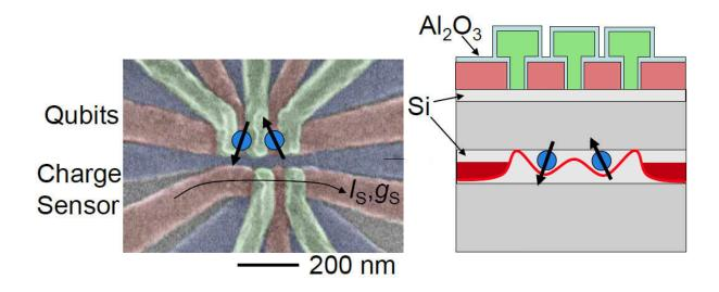
The two-qubit silicon-based gate consists of two electrons (blue balls with arrows) in a layer of silicon (Si). By applying voltages through aluminum oxide (Al2O3)wires (red and green), the researchers trapped the electrons and coaxed quantum behaviors that transform their spin properties into quantum bits of information, or qubits. The image on the left shows a scanning electron
