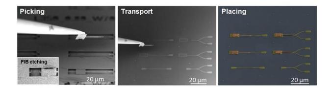
Scanning electron microscope image of the fabricated nanobeam that is suspended by thin tethers that attach it to the bulk substrate. Credit: UNIST
