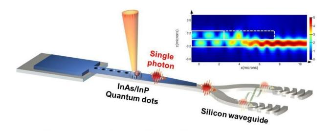
Schematic of the integrated InP nanobeam and silicon waveguide. Credit: UNIST
