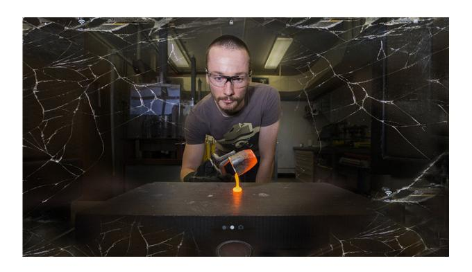
The researchers measured the viscosity of molten glass at more than 1,000 degrees Celsius and the density of the glass when cooled and formed. Credit: Australian National University
