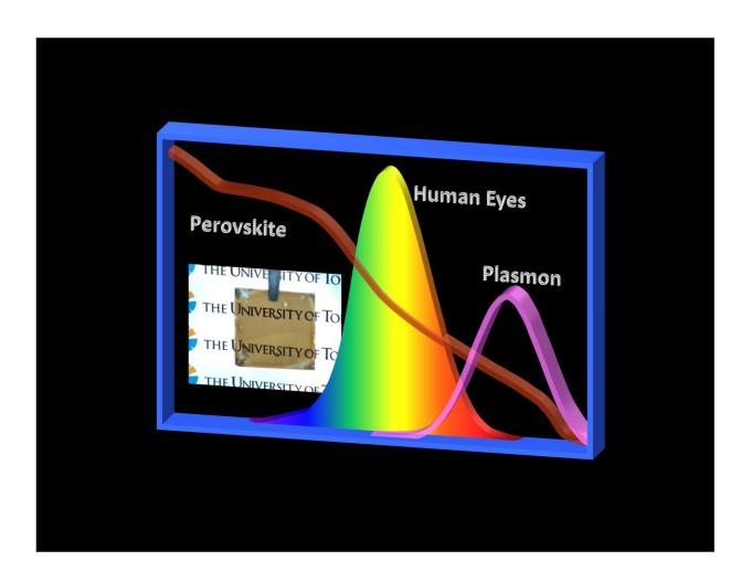
Concept of the visual transparency improvement of the semi-transparent solar cells by considering the human luminosity curve. Credit: University of Tokyo
