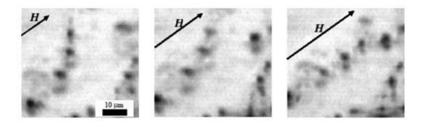
Microphotographs of magnetic polymers with particles forming chain aggregates directed along the magnetic field H. Credit: Andrey Zubarev
