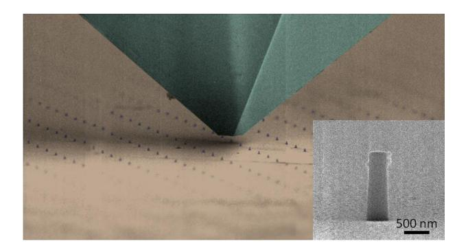
This scanning electron micrograph (SEM) image shows the nanomechanical testing tip passing over the arrays of custom-made nanopillars as it applies pressure to test elasticity and energy storage potential. The inset shows the structure of an individual hybrid nanopillar. Credit: Brookhaven National Laboratory
