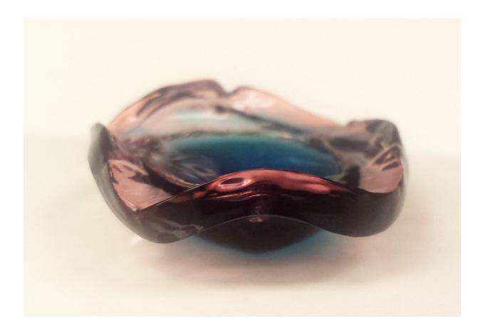
A self-assembled hydrogel bowl with a wavy edge. Blue food dye solution is held in the bowl to demonstrate its structural integrity. Credit: CMU and NTU
