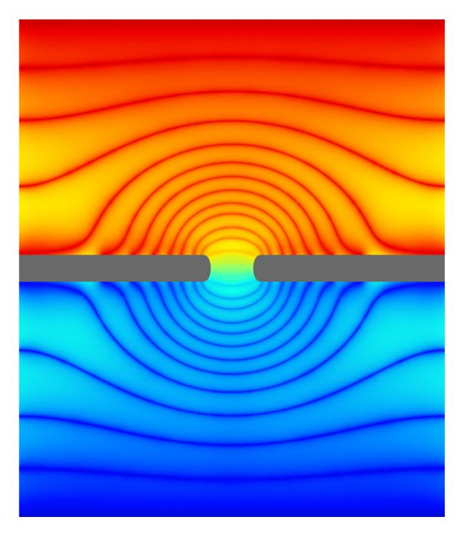
In this simulation, a biological membrane (gray) with an ion channel (center) is immersed in a solution of water and ions. This cross section of a simulation "box" shows the electric potential, the externally supplied "force" that drives ions through the channel. A dazzling pattern emerges in this potential due to the
