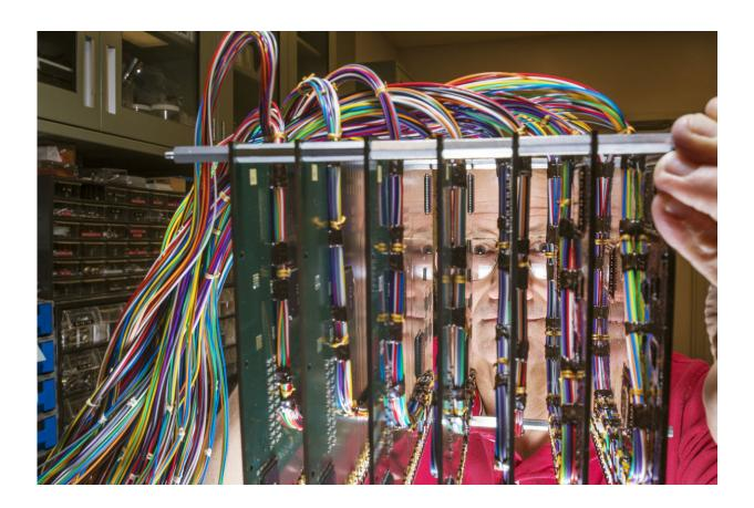
Materials scientist Paul Vianco peers through an experimental setup of printed wiring assemblies used to validate modeling in a Sandia National Laboratories project to study solder failure. Vianco said computational modeling of solder joint fatigue is critical to Sandia's role in life extension programs for nuclear weapons. Credit: Randy Montoya
