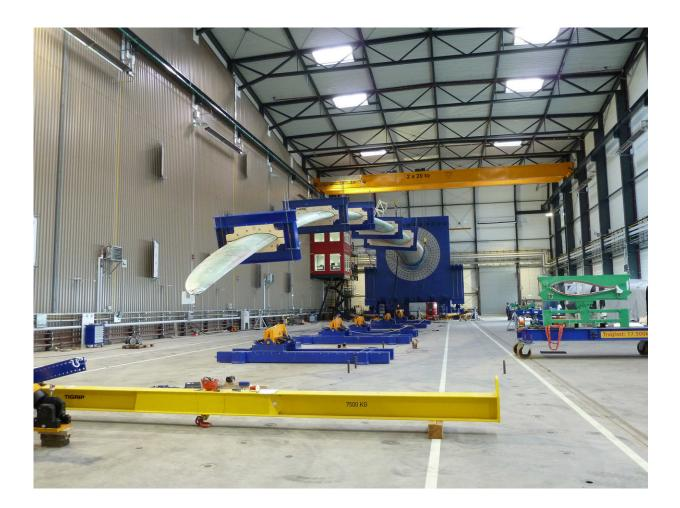
Static testing of the trailing edge of a rotor blade. Acoustic emission sensors were able to detect and locate all defects. Credit: Fraunhofer IWES
