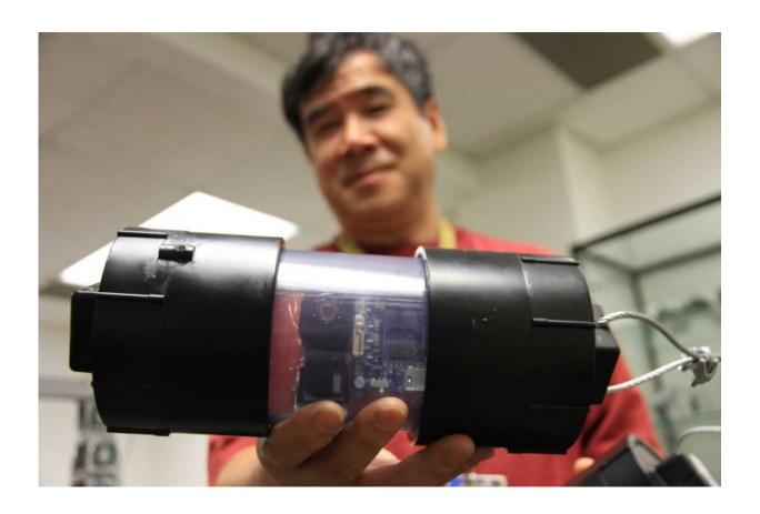
Wei-Min Shen holds an autonomous robot that detects damage in underground pipes. Credit: USC Photo/Caitlin Dawson
